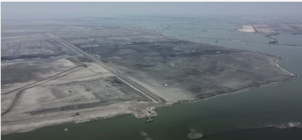
Aerial view of the New Manila International Airport under construction. The dredging works are moving ahead to develop an estimated 1,700 ha of new land. Credit: rexDroneTV.
