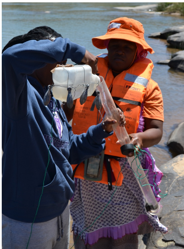
A citizen technician and researcher measure channel turbidity as part of the Tsitsa Project's suspended sediment monitoring programme. Photo: Laura Conde-Aller
